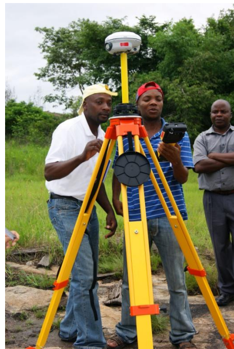
FIGURE 22: PROJECT TECHNICIANS SETTING THE SURVEYING EQUIPMENT (GNSS) DURING THE TRAINING SESSION HELD IN NAMPULA RAPALE DISTRICT, UNDER THE GUIDANCE OF TRIMBLE.
